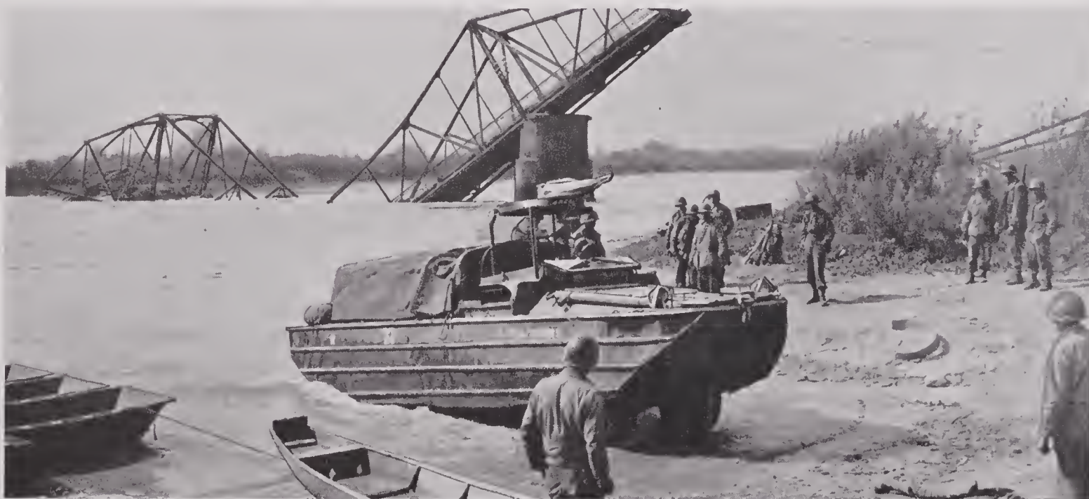
FIGURE 31. DUKW crossing Danube River at Donaustauf, Germany, after other means of crossing were destroyed.
